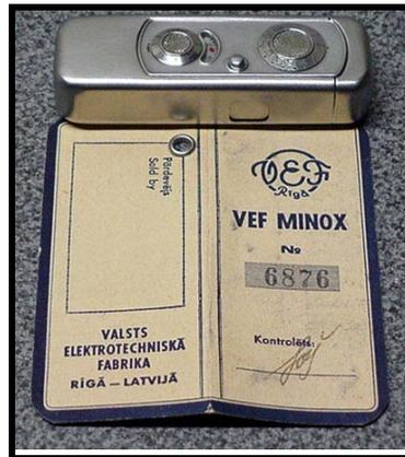
**Riga Spy Camera (Minox).** This small camera (3/4" tall by 3-1/2" wide x 1" deep) uses an 8 x 11 mm negative film with no flash. It can take up to 8 pictures on one roll (and must be changed in a dark room).
